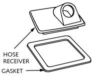
4. Place the hose receiver and gasketin the bowl. Install the Mounting Bracket on the bottom side of the Bowl with four (4) embossed corners facing upward, against the bottom of the Bowl. Secure with four (4) Screws.
