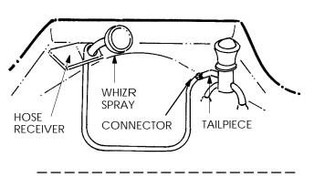
If your bowl *is* equipped with a vacuum breaker, connect one end of the fixture hose to the inlet side of the vacuum breaker. Connect the other end to the fixture tailpiece. Attach the WhizRSpray hose connector to the vacuum breaker outlet.
